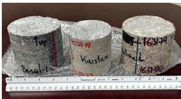
Figure 7: Field cores left to right – Monzonite (Basel-1), Metapelite (Kaisten), and Granite (Schafisheim).
