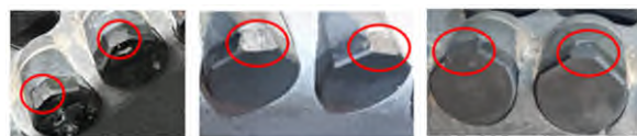
Figure 5: Wear flats are created rapidly, causing ROP to start high and begin to decline. Then, they reach a state where they grow slowly, and ROP is at a near equilibrium. Once the wear flat grows into the stud, the cutter is likely to experience thermal mechanical failure.
