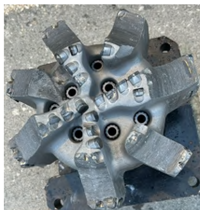
Fig.21: Critical wear progression to the bit body after the integrity of the cutting structure is compromised.
