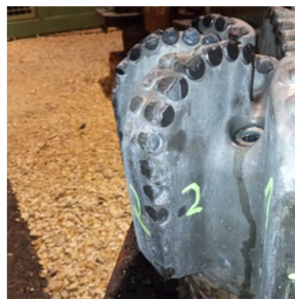
Fig.22: Typical impact damage across the cutting structure. The run was terminated due to low ROP/ineffective cutter engagement.
