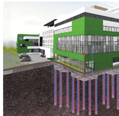
Figure 4: Ambulatory Hospital (Energy Piles) – Oradea
