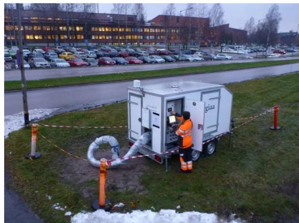
**Figure 5: The thermal response test unit (TRT) of GTK in operation. Photo I. Martinkauppi**
