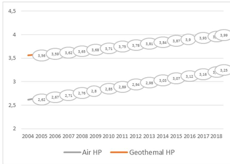
**Figure 7: Calculated SPF of newly installed heat pumps (depending on year of installation)**
