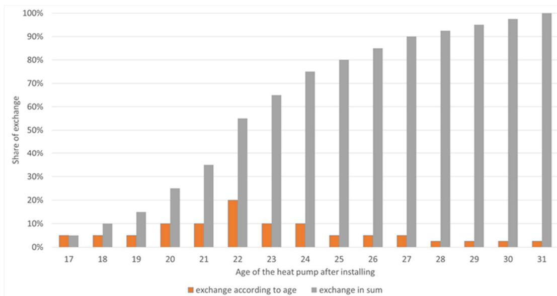
Figure 5: Lifetime of heat pumps – exchange rate of heat pumps according to the age after installation
