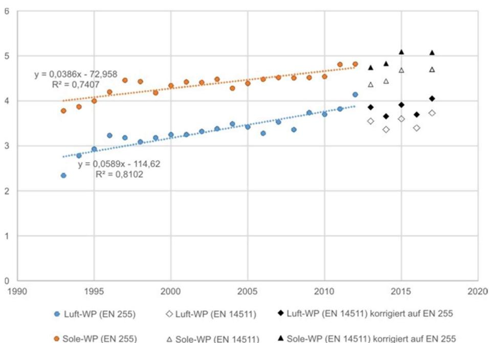
Figure 6: Progression of COP EN 255 [own diagram based on Eschmann, WPZ Buchs 2012 & 2013 and WPZ Buchs 2017]
