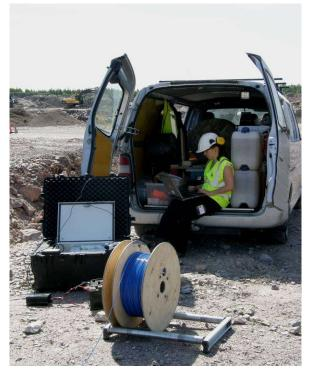
Figure 4: Distributed temperature system (DTS) measurements with fibre optic cable. Photo by I. Martinkauppi.
