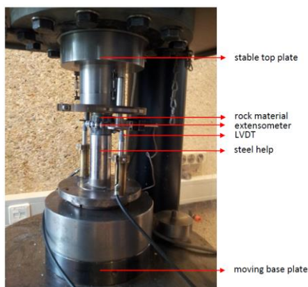
Figure 1: Sample inside the 500 kN loading frame with dummy sample ('steel help + rock material').
