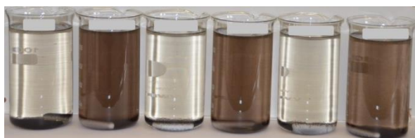
Figure 7: Efficiency of lead sulphide dispersing of different inhibitors after 60 min of settling time (from left to right: blank, polycarboxylate 2, phosphonate 5, polycarboxylate 1, phosphonate 1, polycarboxylate 5). The inhibitor concentration was 50 mg/L.
