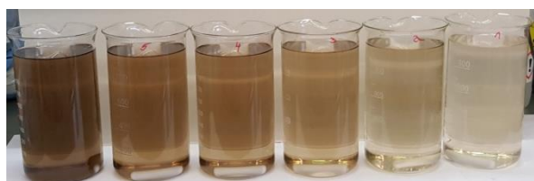
Figure 2: Blank tests with lead sulphide concentrations of 10, 5, 4, 3, 2, 1 mg/L (from left) after 3 min of stirring plus 20 min of settling.
