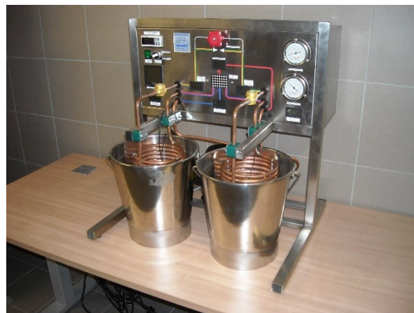
Figure 4: Didactic and research stands of heat pumps.
