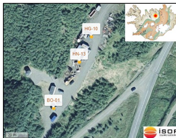
Figure 1. Well HN-13 a non-producer sits between two producing wells used was intended for direct use district heating in Akureyri and nearby communities in North-Iceland.
