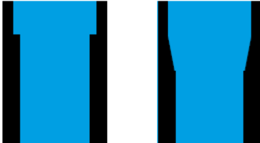
Figure 4: Conical pipe designs still have the disadvantage of a thick-walled area with high hydraulic resistance, reduced thermal conductivity and high material costs.
