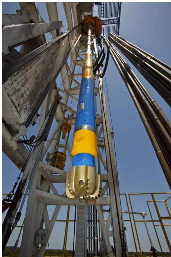
Figure 3: BHGE AutoTrak RSS BHA with PDC bit ready for deployment on a land rig
