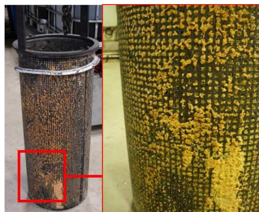
Figure 6: Incompatibility of brine/antiscalants at high temperatures and high calcium concentration at the geothermal power plant Insheim.
