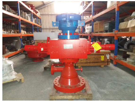
Figure 9: Pressure Control System: fabricated pressure control module, ram BOP and stripper (blue) before final assembly (Thorhallsson, 2017).
