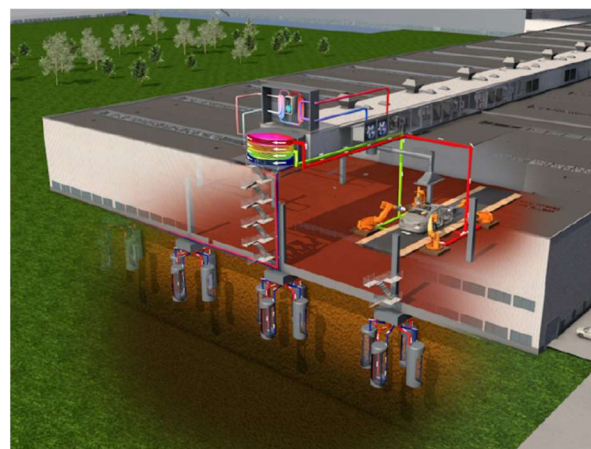
Figure 5: Schematic of one of the sections of the Halle 18 plant; from top: heat pump and air-handling units, layered storage, production hall, energy piles (graph Volkswagen AG).
