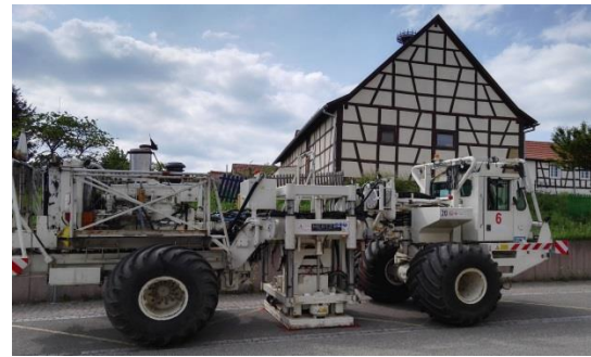
Figure 8: Mertz 26HD-623B (deployed number: 9) - Peak force output 276 kN (62 000 lb).
