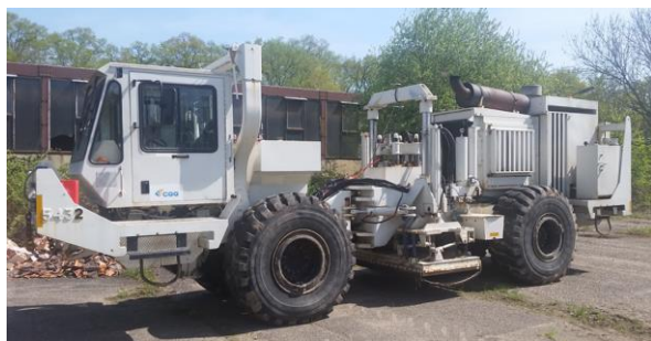
Figure 7: AHV-IV (deployed number: 1) - Peak force output 275 kN (62 000 lb).
