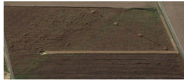
Figure 11: Layout of 6 geophones bunched traces in corn field to allow corn harvesting while recording. (Source Google Maps)
