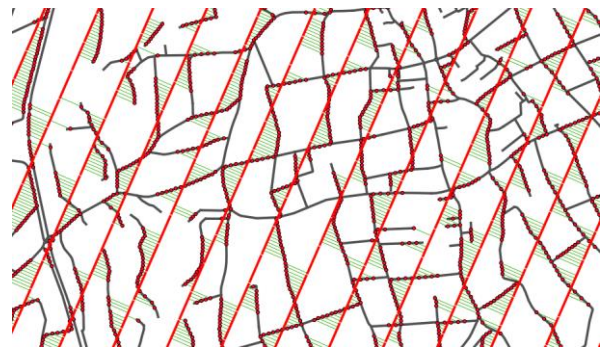
Figure 5 : Deport map of source point positions from theoretical grid to operationally feasible geometry. Red line was the initial 320 m crossline geometry deported (green line) to final positions (red points) on roads (gray line). (Source ESG and CGG)
