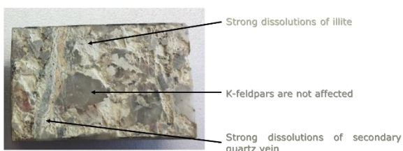
Figure 3: Granite core before and after flooding experiments.
