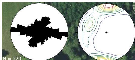
Figure 3: Fracture orientation in the granite of the Saint Pierre Bois quarry
