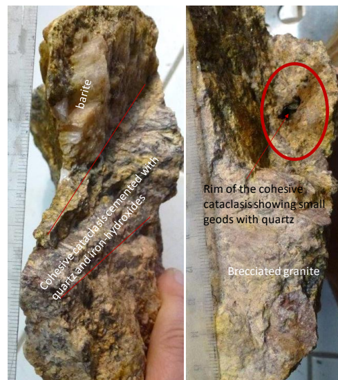
Figure 5: Photographs of the both sides of a same sample of the rim of a cohesive breccia in a major fault showing the porosity of this zone.
