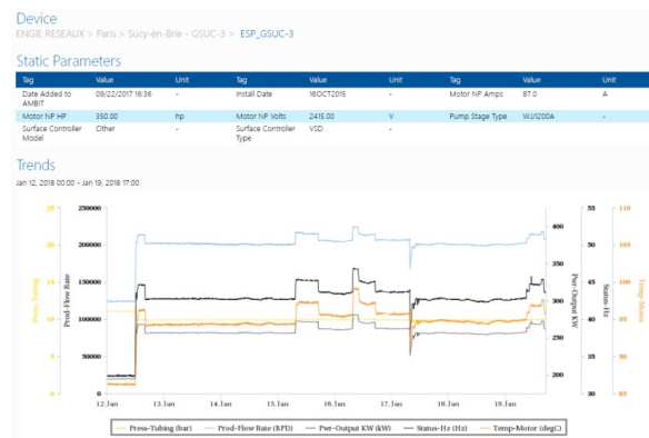
Figure 2: Screenshot of the web application allowing live monitoring of operating wells.
