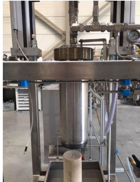
Figure 1: Photo of 'iBOGS mini' pressure vessel being used for jetting experiments under pressure controlled conditions.
