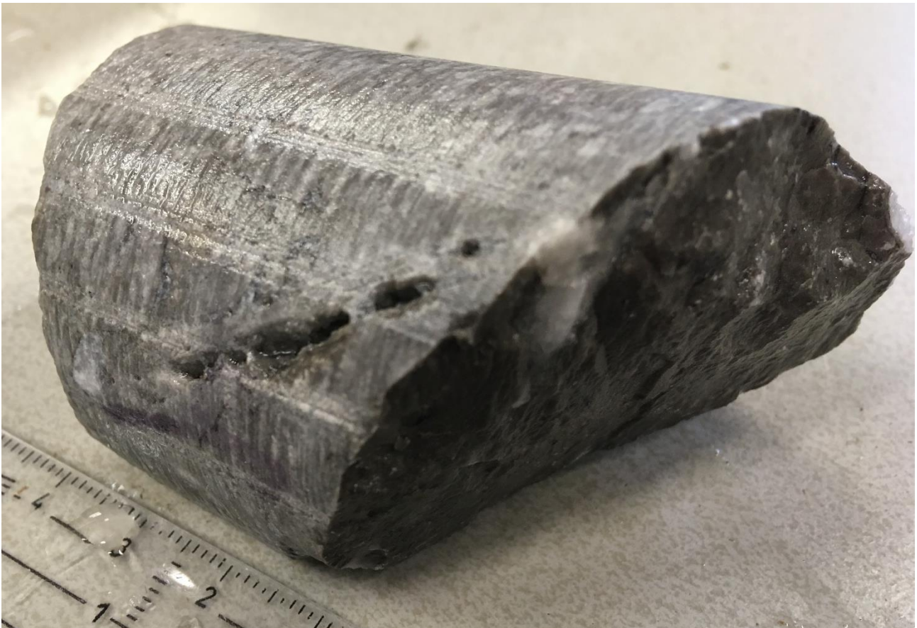
Figure 3 Example of a partially open vein in a core samples of the Heibaart DZH1 borehole, at a depth of 1178m. This vein is partially cemented by calcite. The numbers on the scale represent cm.
